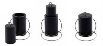
Bucket (external measures): h = 60 mm; d = 41 mmCylinder: h = 50 mm; d = 30 mm
