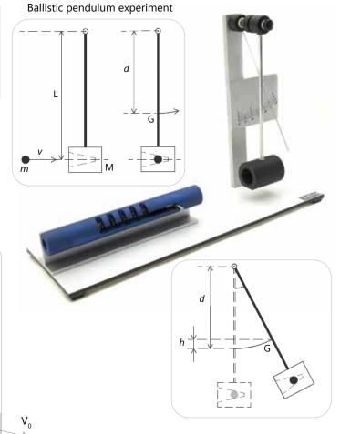
The launching system is removable and suitable to verify the initial speed of the projectile, according to the laws of parabolic motion; this allows to compare the result with that one obtained by performing the inelastic collision experience.
